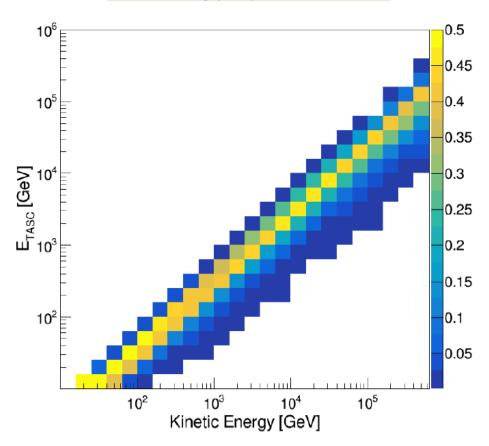
The energy resolution of helium is 30-40%. Therefore, we apply Bayes unfolding to reconstruct energy.
