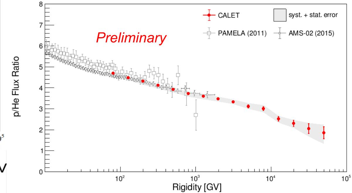
The relative flux of proton to helium decrease with rigidities, and no clear structure is not seen in the flux.
