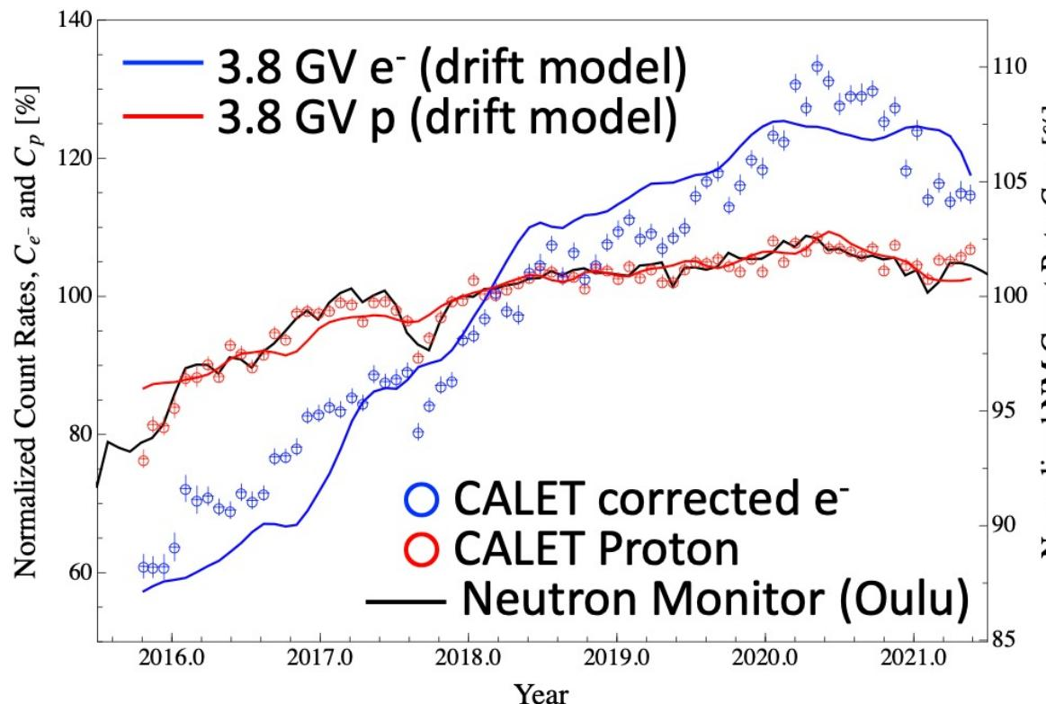
Correlation with count rate of CR protons/corrected  $e^-$  and HCS tilt angle
