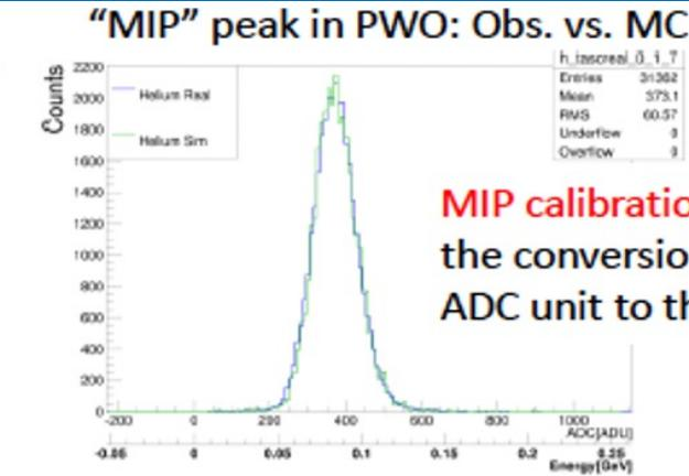
**MIP calibration** determines the conversion factor from ADC unit to the energy
