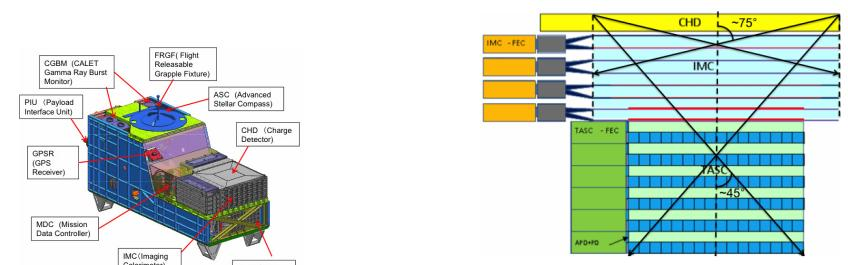
Figure 1(a): CALET instrument package detailing location of various CALET subsystems.
