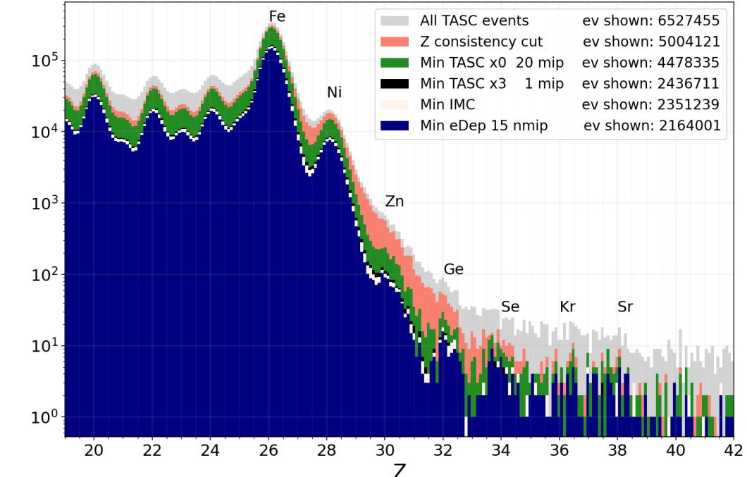
Figure 4: A charge histogram showing what each successive cut on the TASC data-set does step-by-step from a charge consistency cut that requires both x and y layers to be within 2.00%, cuts on multiple layers of the TASC and IMC, as well as a minimum TASC energy.
