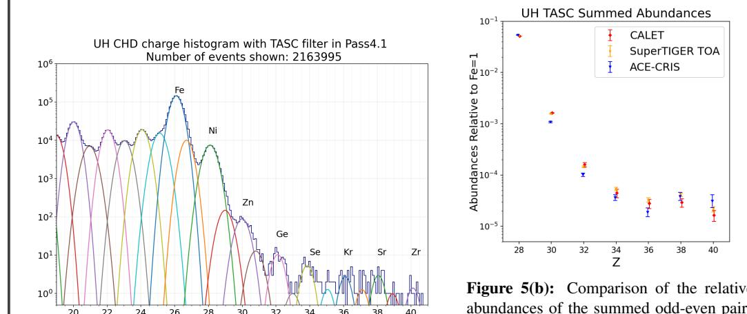
Figure 5(a): UHCR TASC analysis histogram with multiple gaussian fitting, bin size in 0.1 units of charge.
