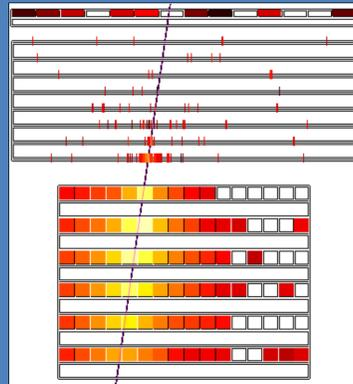
Figure 1. Event viewer image of a gamma-ray candidate in the CALET calorimeter.
