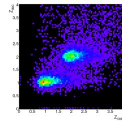
Proton/helium separation using CHD/IMC charge
