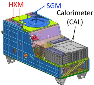
Figure 2. Schematic image of the CALET. The two HXMs and SGM are mounted on the upper side of the CALET. CAL is a main high energy calorimeter.
