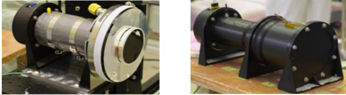
Figure 1. Pictures of the HXM and SGM. SGM is BGO covered by a housing made of aluminum, HXM is LaBr<sub>3</sub>(Ce) with a Be window to detect low energy X-rays.
