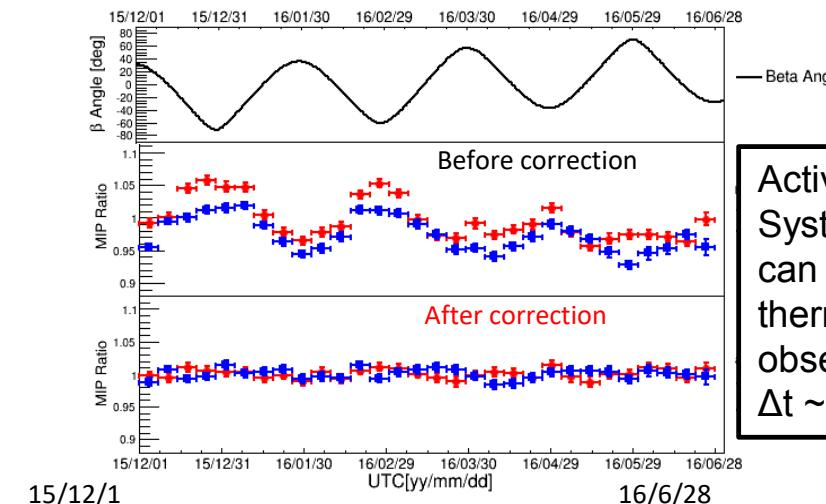
Active Thermal Control System (ATCS) on ISS can provide very stable thermal condition during observations:
