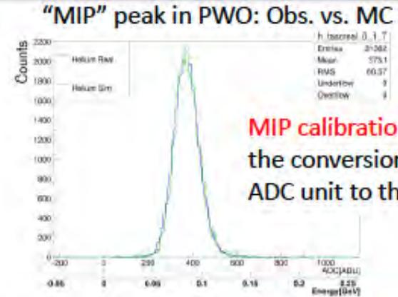
MIP calibration determines the conversion factor from ADC unit to the energy
