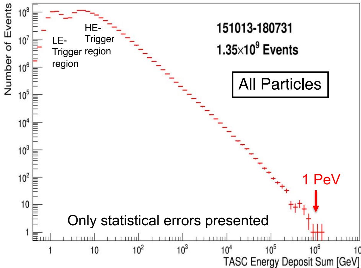
The TASC energy measurements have successfully been carried out in the dynamic range of 1 GeV – 1 PeV.
