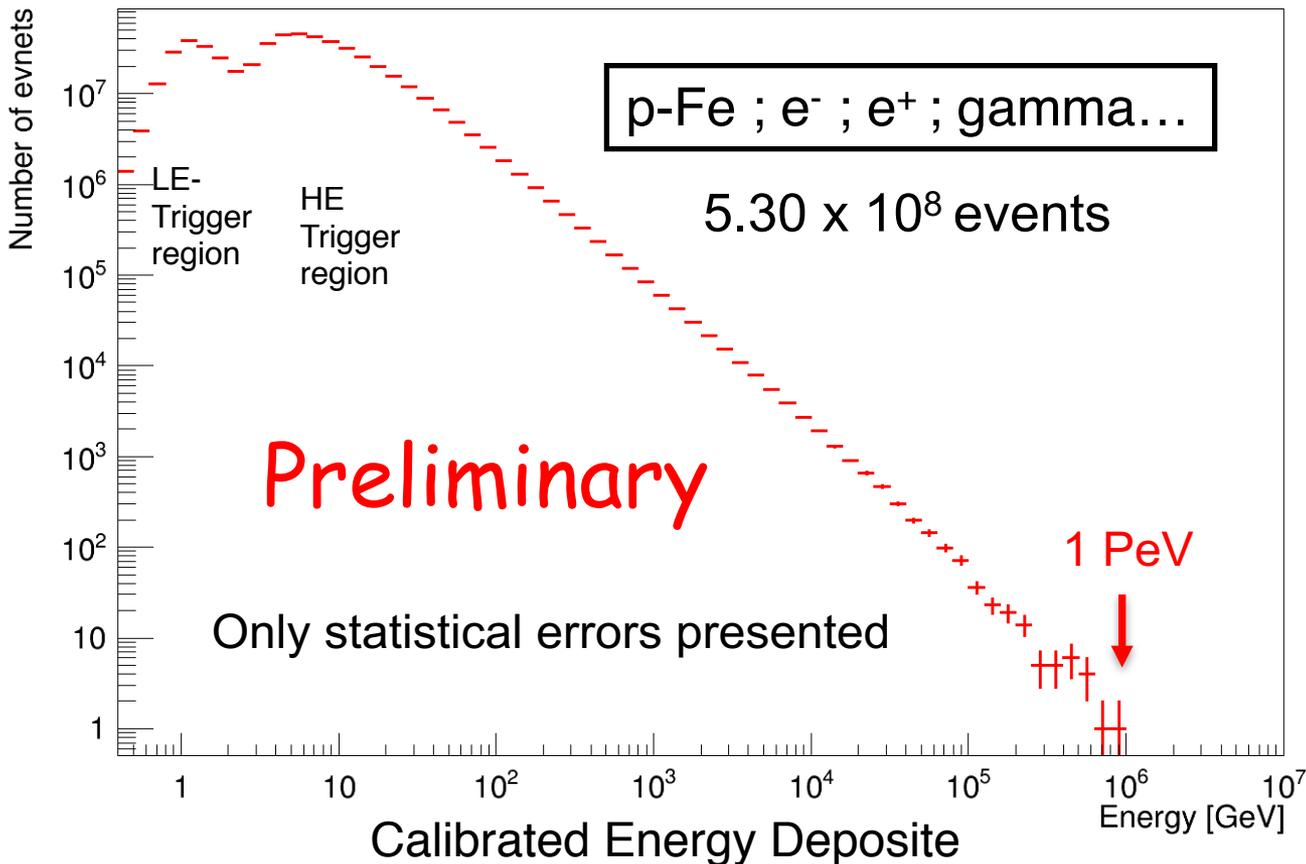
The TASC energy measurements have successfully been carried out in the dynamic range of 1 GeV - 1 PeV.
