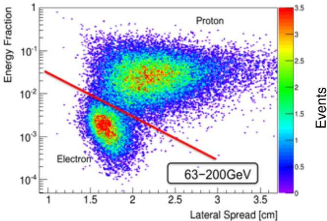
**Simulation:** e/p at 1TeV  $\sim 1.3 \times 10^5$  with  $\sim 90\%$  efficiency for electrons
