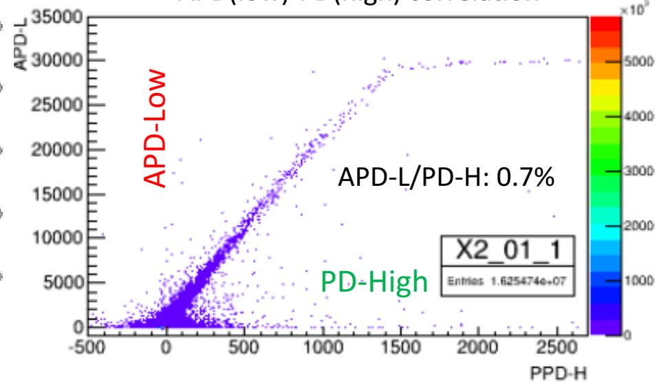
The correlation between adjacent gain ranges is calibrated by using in-flight data in each channel. The linearity has been calibrated by using **UV laser irradiation** on ground:
